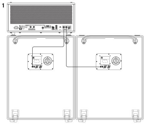
In example **1** above, a speaker cable with 1/4" ends connects from one speaker output of the amplifier to the speaker input of the Ampeg SVT-410HLF cabinet. An additional cabinet may be connected by attaching another speaker cable from the remaining 1/4" speaker output of the amplifier to a speaker input of the next cabinet.
